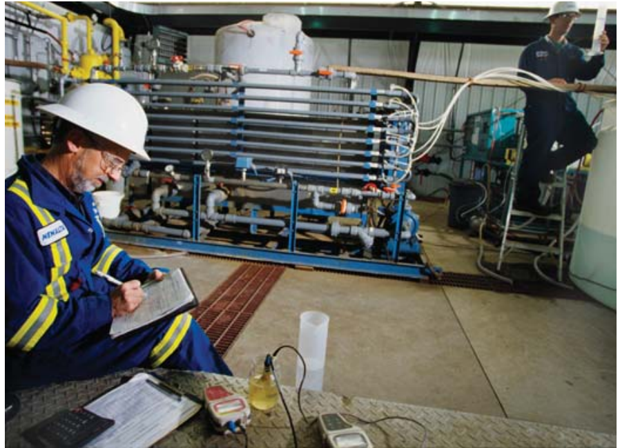
Pilot testing membrane filtration technology for recycling of oilfield wastewater. Author is pictured in foreground.
