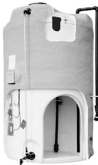
Primary tank dome design extends over containment area to eliminate the entrance of rainwater. Shown with convenient top entry fill and suction lines. Flat recessed area available for optional bottom outlet fittings.
